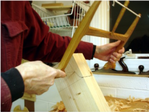
Cutting the top shapes. Turning saw uses a 10 TPI by 1/8" blade. Workpiece is 3" thick.
