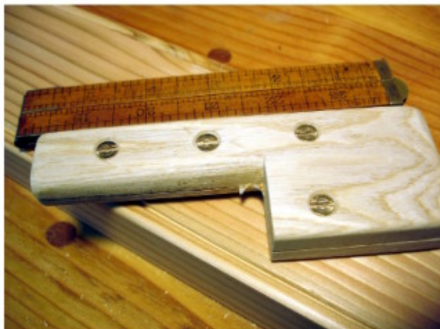
Scratch stock has 2 registration surfaces, one flat, the other rounded.
