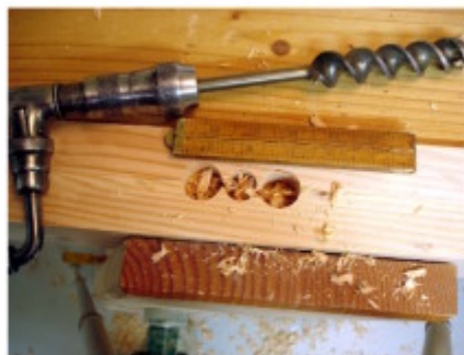
3 holes: 1 inch on each end and 3/4 inch in the middle.
