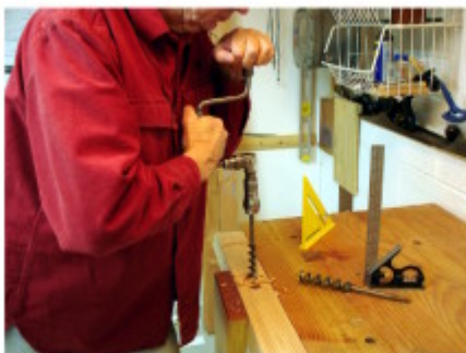
Drill using numerous sighting references for vertical. Rules, corners, window frames, etc.
