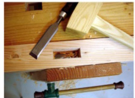
Work half way through. Then, turn the workpiece and do the other half.
