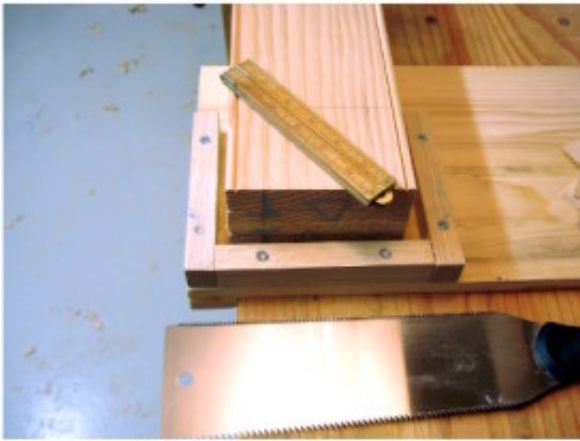
Tenon cutting jig, a modified bench hook.
