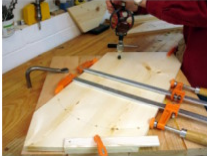
Add a layer of 1x pine to each side. Glued and screwed.
