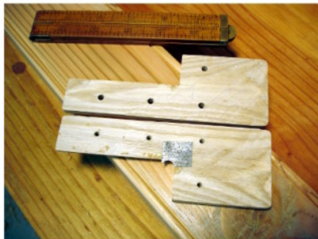
Opened, we see the metal scratch blade.
