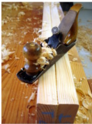
A #40 scrubs down the ridges. Thick, 1/16" - 1/8" shavings.
