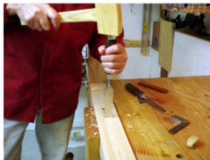
Remove waste with bench chisels.
