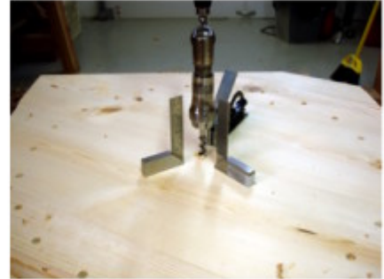
Drill 1/2 inch hole carefully.
