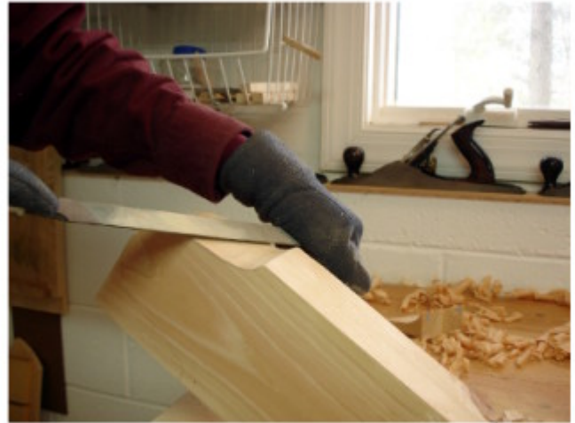
A cabinet maker's rasp brings the shape to the line. Raking daylight from the window helps.
