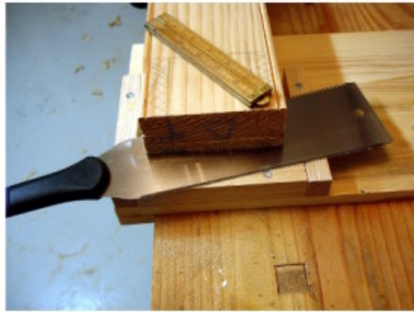
Cutting with the ryoba. Saw to the right. Saw to the left, then do-sa-do down the middle.
